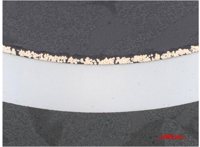
Figure 6: Steel sleeve bearing with copper and Teflon coatings, as-polished, 2.5X objective, Brightfield
