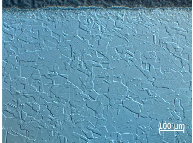
Figure 8: Inconel X750 wire, as-polished, 20X objective, C-DIC
