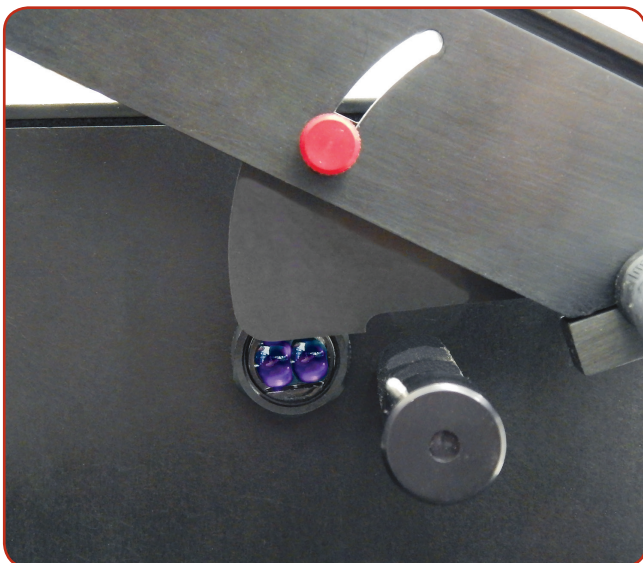
Optical shut-off sensor with adjustable stop
