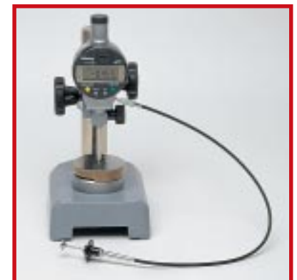
Verify thickness with #120-30010 Digital Measurement System
