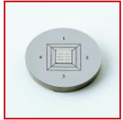
IC mounted on fixture (sample size: 14mm x 14mm)
