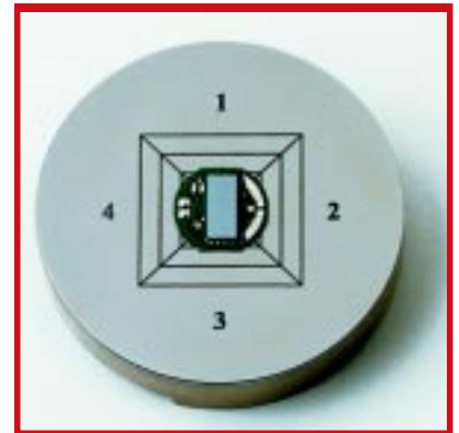
Flip Chip package mounted on fixture
