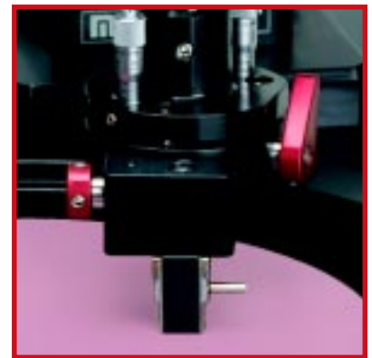
Unencapsulated electronic package mounted on paddle
