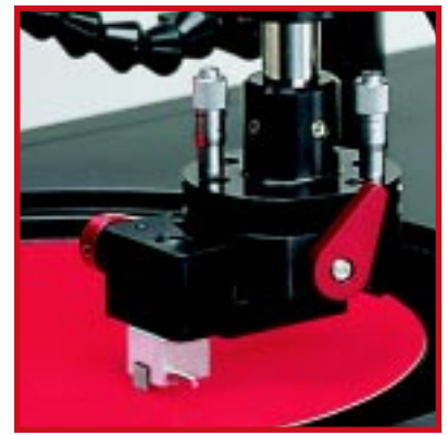
IC Die mounted on cross-sectioning paddle
