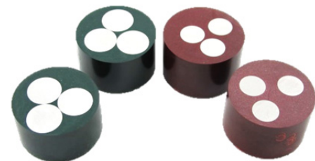
Figure 2: Aluminum rods (green) and steel rods (red) were mounted in phenolic.
