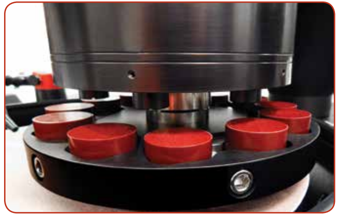
PH-6™ central force configuration: one (1) central piston applies force to up to twelve (12) mounts (1.25" mounts shown).
