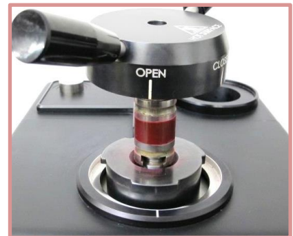
Figure 2: Remove the mount after the cycle has finished.
