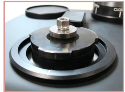
Figure 1: Place the sample in the center of the die.
