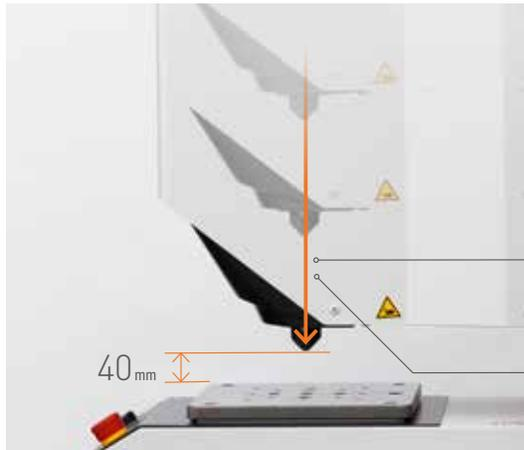
First Mitutoyo hardness testers ever to be equipped with moving heads (the head moves at a speed of 10 mm/s within a 210 mm range).
