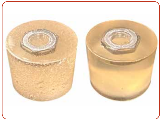
Acrylic samples mounted without & with pressure chamber
