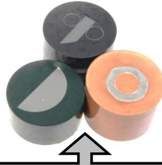
If the sample needs to be removed from the mount, it may be possible to remove it by sectioning away excess material with a plated rim diamond blade and then chiseling away the remaining mounting material.
