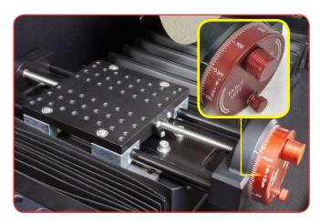
The X-axis indexing tables allow quantitative positioning for sectioning in precise locations. Two resolution options are offered: 25  $\mu m$  (coarse) and 5  $\mu m$  (fine). Coarse positioning is more applicable for metallurgical sectioning applications, where fine positioning is more suitable for tight geometry requirements usually found in microelectronic failure analysis and dicing applications.
