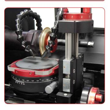
The dicing rotation stage (shown mounted on #5-5730 Z-axis stage and #5-5325 fine indexing table) allows 360° rotational positioning of flat substrates. Samples are mounted to the borosilicate glass insert using wax, which is secured with setscrews for quick attachment and removal. It can be mounted directly to the indexing tables, or to the Z-stage to control cutting depth.
