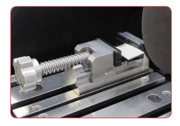
Made of hardened 17-4 stainless steel, the quick-slide vise features a lead-screw that disengages for quick and easy operation. Removable delrin inserts (included) are ideal for holding brittle or delicate samples. The vise mounts directly to the indexing or T-slot tables.
