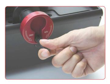
Manual Y-axis sample advancement using the hand wheel provides additional flexibility in positioning and feeding. The wheel is utilized to slowly feed delicate samples into the blade for minimal damage, allowing the user to "feel" the sectioning operation or to quickly position the sample prior to sectioning. It is also convenient for blade dressing.
