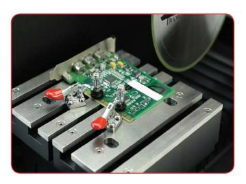
Flat samples up to 0.25" (6 mm) thick can easily be secured to the T-slot table with these height adjustable clamps.
