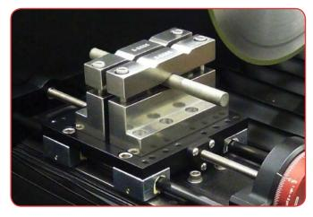
These stainless steel saddle clamps provide single or dual clamping for cross-section cuts. They mount directly onto the indexing tables and can be spaced at different widths for versatility. V-notches on both sides of the clamp hold parts securely in place.
