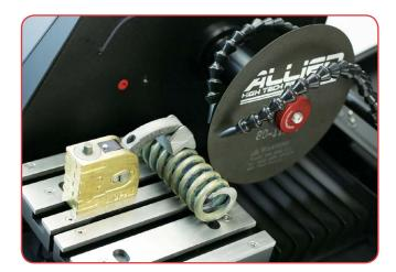
The vertical adjusting clamp can be positioned in any orientation throughout the T-slots in the table. The height adjustable lever allows various size samples up to 2.25" (57 mm) to be secured. Interchangeable pads allow handling of a variety of sample shapes. One (1) angled pad and one (1) flat pad are included.
