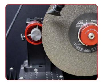
The rotational cutting attachment, which mounts directly to the indexing or T-slot tables, enables sample rotation during a cut. Its benefits include:
