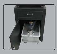
Cabinet - Internal View with External Coolant Reservoir (5-5700-ER)
