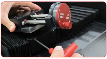
The TechCut 5's unique design allows the use of either a T-slot table or X-axis indexing table, which are easily and quickly changed to support a wide range of fixture configurations.
