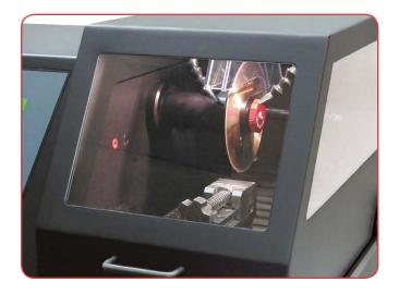
LED illumination inside the cover allows easy observation of the sectioning process through the large viewing windows.
