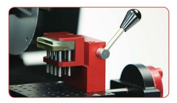
The cam-lock fixture adapter offers a quick and convenient method for securing and detaching the #15-1045 multipurpose fixture to the indexing tables. The sectioned sample can then be transferred without disturbing orientation directly to the MultiPrep™ for grinding/polishing on the same plane.
