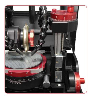
The Z-axis stage (shown mounted on #5-5325 fine indexing table with #5-5540 dicing rotation stage) allows vertical positioning of the sample relative to the blade. It provides 2" (51 mm) of travel with 5  $\mu$ m increments. The platform has a 0.5" center-threaded mounting interface for stage/fixture positioning versatility, and it mounts directly to the indexing tables.
