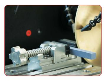
Loaded/clogged blades can easily be dressed to resume optimal cutting performance. The quick-slide vise or vertical clamp is used to hold the dressing stick, and then indexed manually into the blade using the hand wheel.
