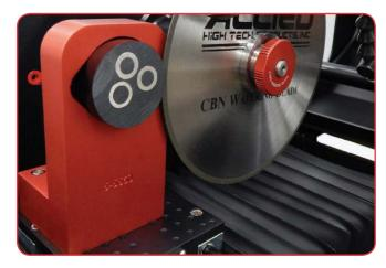
The teardrop holder secures various sized mounts from 25 mm to 2" diameter. It is mounted to the indexing tables for precise location sectioning, and positions the mount at the center of the blade.
