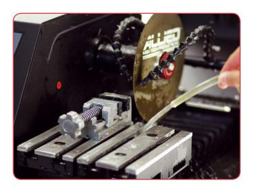
The wash-down hose is used to clean the cutting compartment. A quick-connect fitting on the end of the coolant nozzle bridge allows the hose to be connected for temporary use and disconnected for storage.
