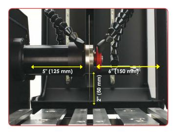
With a 5" (125 mm) clearance to the left-hand side of the blade and 6" (150 mm) to the right side, long and/or large parts are easily accommodated.
