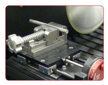
During the cutting process, adaptive force control optimizes the feed rate through the sectioning process, allowing the operator to select force or feed as the preference for control.
