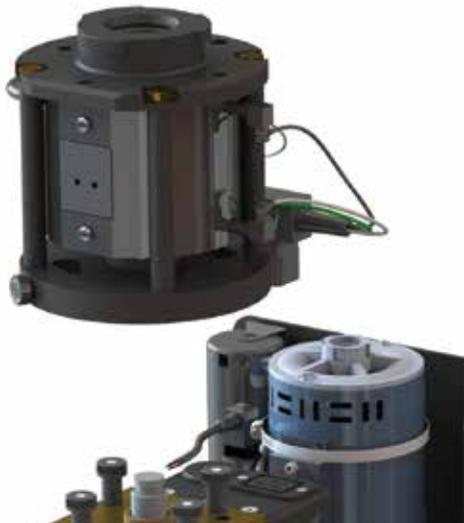
Remove and Replace Mold Assembly
