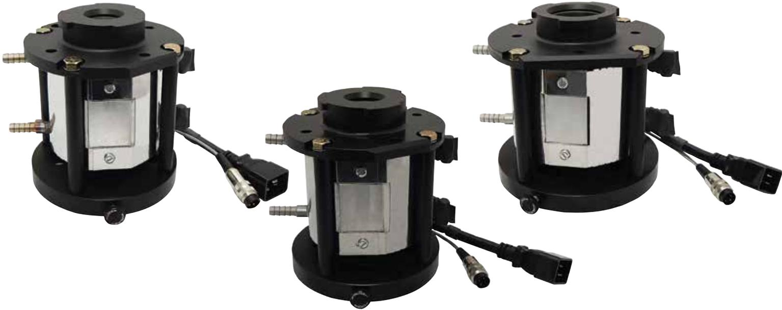
A range of mold/heater assemblies are available to accommodate various size samples. They may be changed from 25 mm through 2 inch, and include a duplexing spacer, allowing up to two mounts per cycle to be produced at one time. The new coiled heating and cooling lines within the cast housing and thin-walled cylinders allow quick and efficient cycling.
